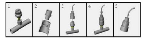
1. Install the remote sensors into the system plumbing (use 3/4" hex to tighten")
