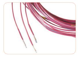
abuses normally encountered in Validation. Type T wire and probes provide the highest level of accuracy when used from -200°C to 400°C. The Teflon coated wire is rated for continuous use at 200°C with a peak rating of 260°C, while our Kapton coated insulated wire will withstand use up to 400°C.
