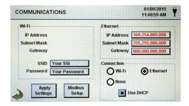
Ethernet Communication IP Address, Subnet Mask, & Gateway The particle counter can support Ethernet RJ-45 connection to a network for communications. Enter in the IP address for the device for your network the Subnet mask and gateway for your router. A numeric keypad will be displayed for entering these values.
