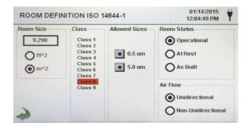
Each report standard has a Room Definition page that allows for information to be input defining the output of the generated report. Room size is input in square feet or square meters. The ISO class of the cleanroom being tested is selected, and the allowable sizes may be included or excluded in the report. The Room Status is selected as being Operation, At Rest, or As Built per the standard specification requirements. Airflow is recorded as being Unidirectional or Non-Unidirectional.
