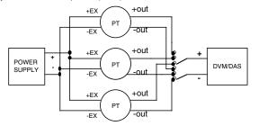
NOTE: The shield is internally commoned to the case and pressure port of the transducer. When the shield is connected to ground the case and pressure port of the transducer will also be commoned to that ground.
